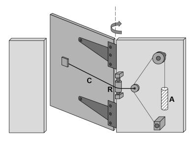
The pulley system raises weight  ${\bf A}$  when the gate is opened. When the gate is released,  ${\bf A}$  falls. The horizontal cable  ${\bf C}$  passes over pulley  ${\bf R}$ . The tension in cable  ${\bf C}$  causes the gate to close.
