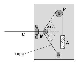
Pulleys  ${\bf P}$  and  ${\bf M}$  are frictionless so that the tension in the rope attached to  ${\bf A}$  is equal to the weight of  ${\bf A}$ .
