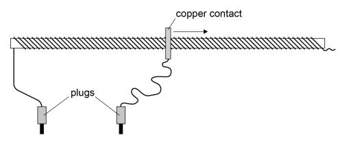
Two plugs connect the variable resistor into the circuit. A moveable copper contact is used to vary the length of wire in series with the lamp.
