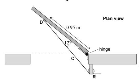
The tension in the horizontal cable  ${\bf C}$  is now 41 N.
